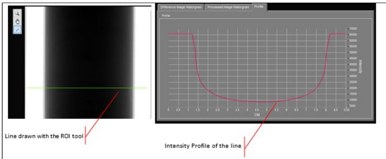
Figure 25. Example of ROI tool used on a raw image and the resulting intensity profile.
