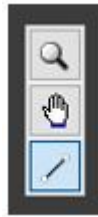
Figure 24. ROI tool available in the image processing utility. The histogram or line profile will be displayed when the ROI tool is used. A line will produce a line profile. A box will produce a histogram.
