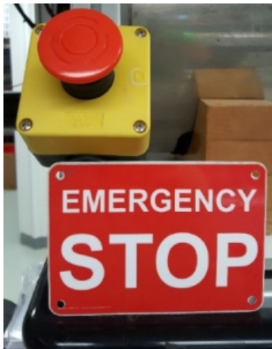
Figure 40- Hardware Emergency Stop Button
