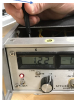
Figure A5: Zeroing the fluxgate by A) fine tuning or B) coarse tuning.
