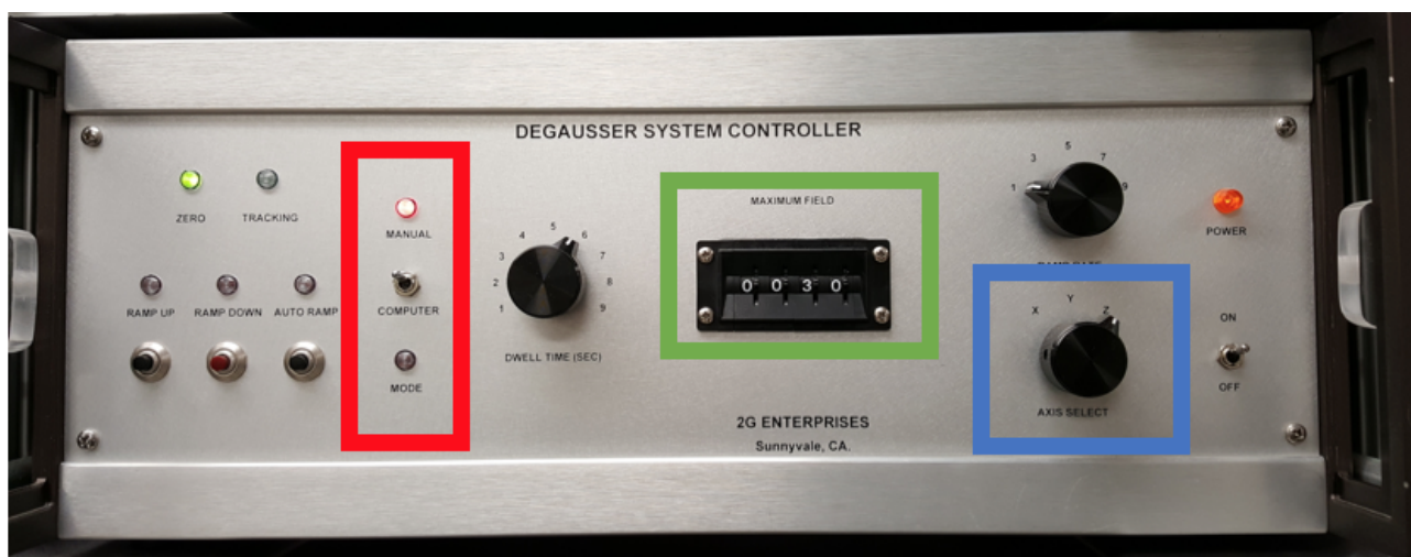
Figure 74 Degausser Control unit. Red box indicates the toggle switch for switching to manual mode.
