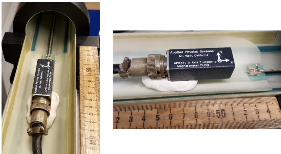
Figure A5: Fluxgate Magnetometer probe positioned in the section half boat. Center the probe in the bore.
