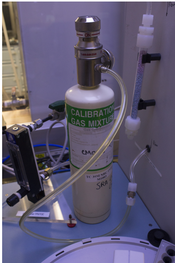
Figure 9: Setup of the IR cell calibration
