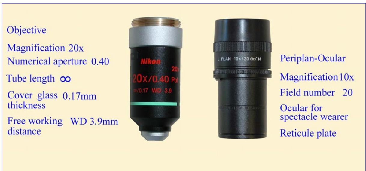
Figure 1.2-2: Objective (Example: Nikon CFI Achromat 20x P) and ocular (Example: Leica Periplan with reticule plate)
