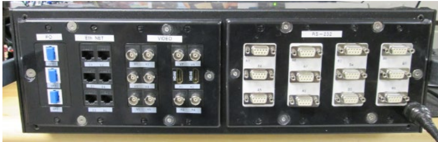
Figure 3. Surface Multiplexer Box.
