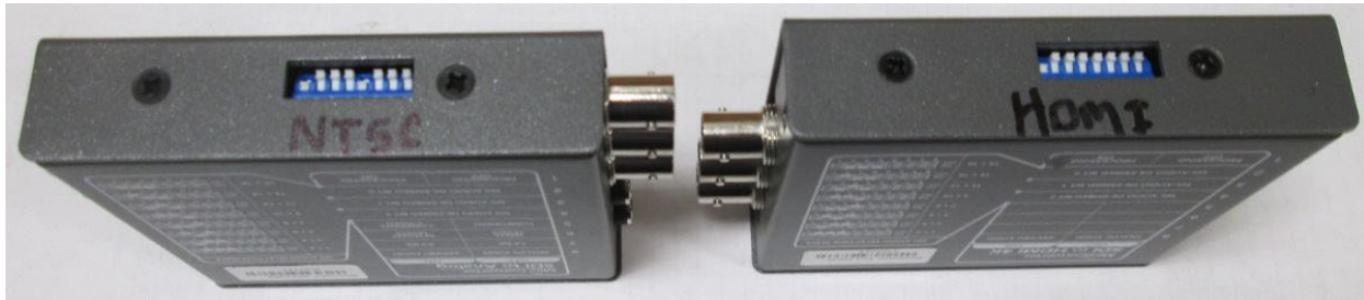
Figure 12. NTSC 1 & 5 ON (Left) and HDMI 1 ON Dipswitch Settings (Right).
