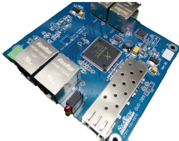
Figure 10. SVS-209 Gbit Ethernet Converter.
