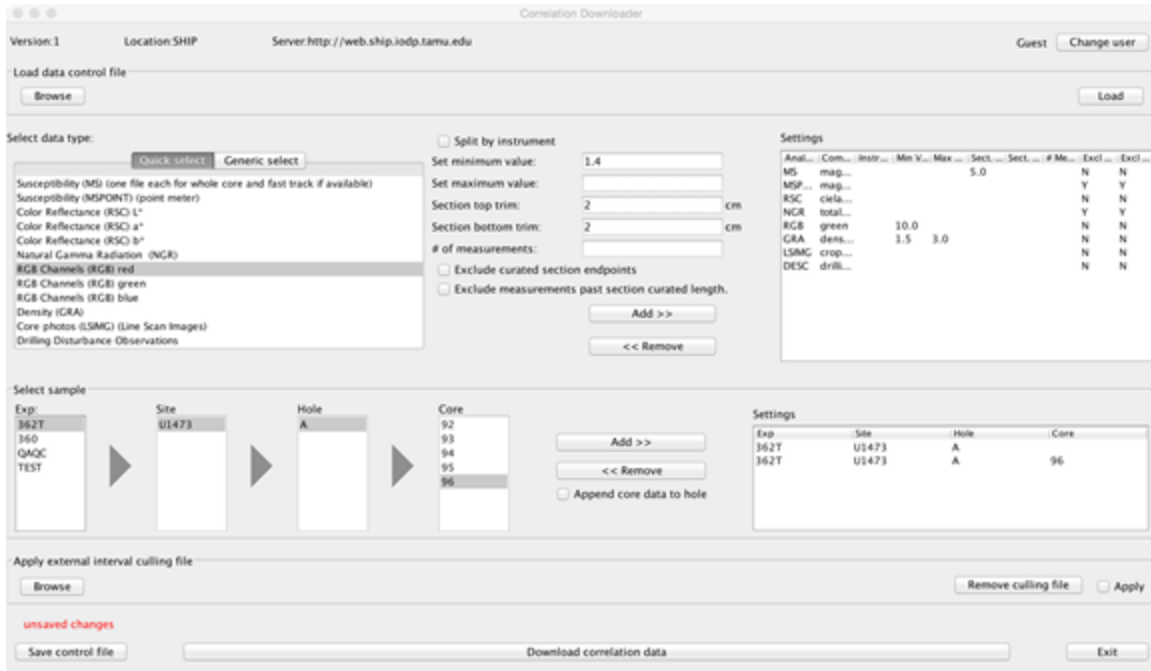
Figure 2-1. The Correlation Downloader application is a single-window Java interface allowing you to specify all aspects of data types, filters and modes of download as you proceed from top to bottom and left to right.
