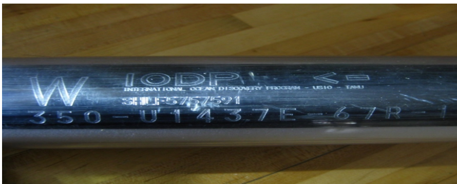
Figure 5. Full format engraving for a section half.
