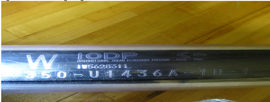
Figure 6. Full format engraving for an interstitial water whole round sample.
