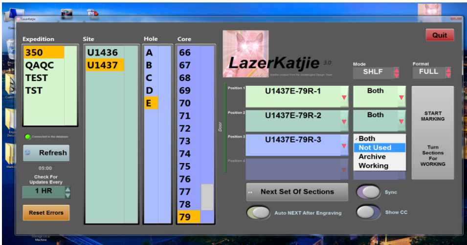
Figure 4. Specifying Mode: Archive, Working, Both or if the position is Not Used from drop down menu.
