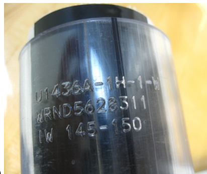
Figure 7. Small Format Engraving when Mode is set to a) Section Half or b) Whole Round. Note that Small format is only used for sections that are too small for the Full format or whole round samples.
