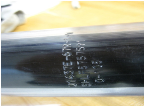
Figure 7. Small Format Engraving when Mode is set to a) Section Half or b) Whole Round. Note that Small format is only used for sections that are too small for the Full format or whole round samples.
